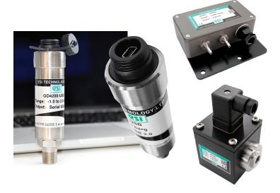
The ESI **GD4200-USB**© Digital Pressure Transducer has been designed to measure, analyze and record pressure directly on your computer. It allows the user to measure up to 16 pressure inputs simultaneously and easily create customized test certificates. Sample rate up to 1,000 Hz (1,000 readings per second).
