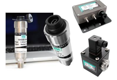
The ESI **GD4200-USB**© Digital Pressure Transducer has been designed to measure, analyze and record pressure directly on your computer. It allows the user to measure up to 16 pressure inputs simultaneously and easily create customized test certificates. Sample rate up to 1,000 Hz (1,000 readings per second).
