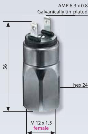
0168 Diaphragm pressure switches with spade terminal
